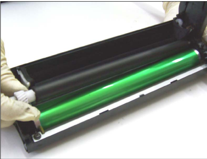
15. The developer roller should come out easily.
