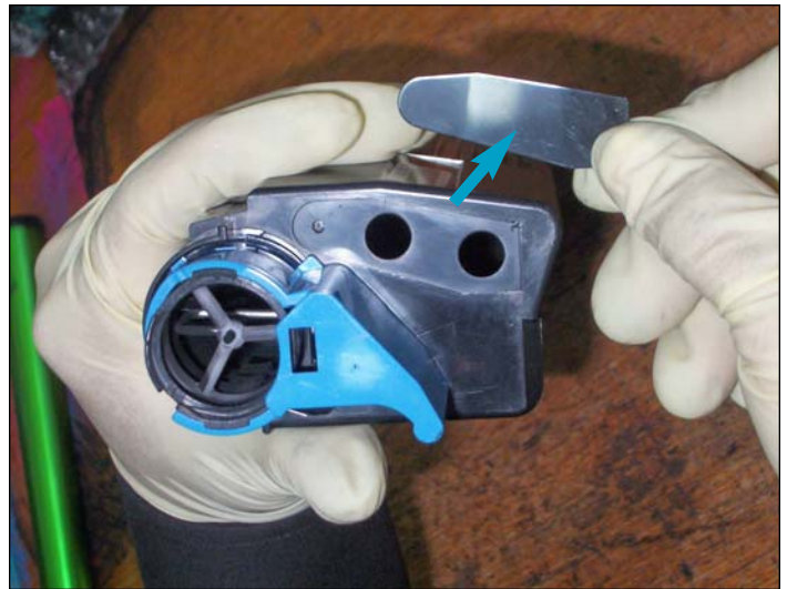
28. Using a thin needle or small hook tool, pry off the plastic adhesive tab from the waste hopper openings (two holes) shown. This is where the waste toner will dump out during cleaning.
