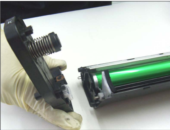
17. The large end cap should easily come out.
