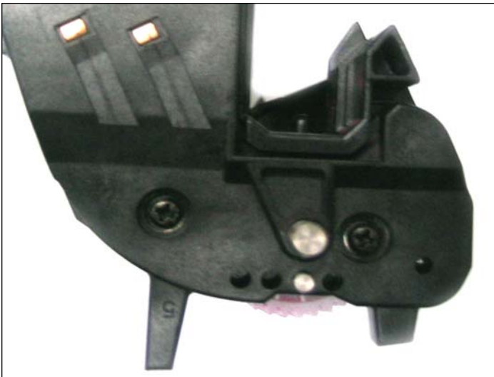
11. Close-up view of small end cap with two screws.
