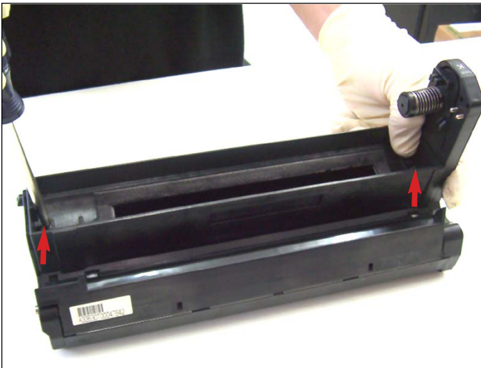
3. Separate the drum unit from the plastic cover by first removing the two screws as shown.
