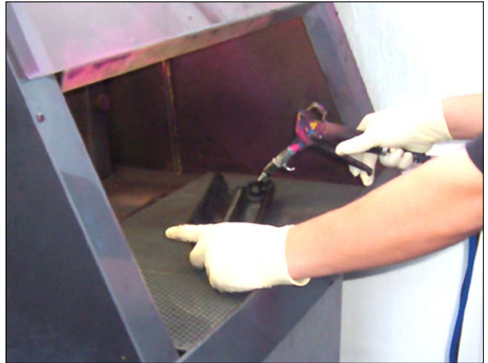
24. Clean using air pressure. Reassemble when done.
